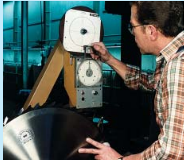
Straightening and tensioning
