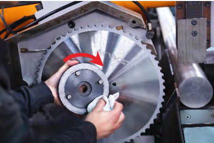
3 The cover of flange must be free from scratches and wiped clean.
