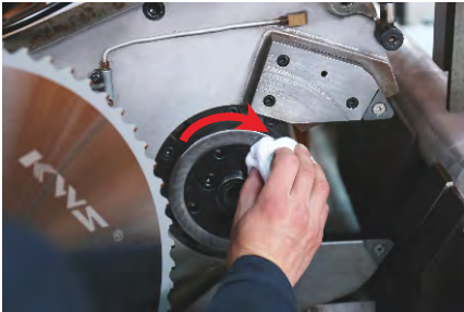
2 The flange must be free from scratches and wiped clean.
